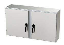
Saginaw Enviroline series enclosure, NEMA 3R/4/4X/12/13, 24 x 42 x 10in (HxWxD), wall mount, 304 stainless steel, #4 brush finish, 2-door, 3-point keylocking/padlocking combo handle.
