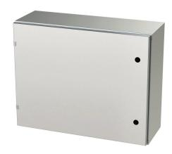
Saginaw Enviroline series enclosure, NEMA 3R/4/4X/12/13,  $24 \times 30 \times 10$ in (HxWxD), wall mount, 304 stainless steel, #4 brush finish, single-door, 1/4-turn semi-flush latch.
