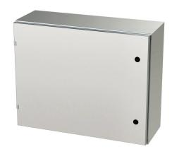
Saginaw Enviroline series enclosure, NEMA 3R/4/4X/12/13, 24 x 30 x 10in (HxWxD), wall mount, 316L stainless steel, #4 brush finish, single-door, 1/4-turn semi-flush latch.
