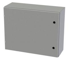
Saginaw Enviroline series enclosure, NEMA 3R/4/12/13, 24 x 30 x 10in (HxWxD), wall mount, carbon steel, ANSI 61 gray, powder coat finish, single-door, 1/4-turn semi-flush latch.
