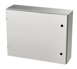
Saginaw Enviroline series enclosure, NEMA 3R/4/4X/12/13,  $24 \times 30 \times 8$  in (HxWxD), wall mount, 316L stainless steel, #4 brush finish, single-door, 1/4-turn semi-flush latch.
