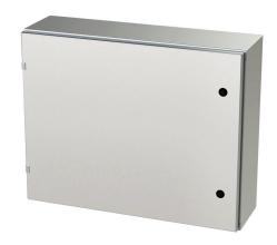
Saginaw Enviroline series enclosure, NEMA 3R/4/4X/12/13, 24 x 30 x 8in (HxWxD), wall mount, 316L stainless steel, #4 brush finish, single-door, 1/4-turn semi-flush latch.
