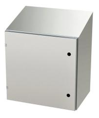
Saginaw Enviroline series enclosure, slope top, NEMA 3R/4/4X/12/13,  $24 \times 24 \times 16$ in (HxWxD), wall mount, 304 stainless steel, #4 brush finish, single-door, 1/4-turn semi-flush latch.
