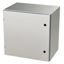
Saginaw Enviroline series enclosure, NEMA 3R/4/4X/12/13,  $24 \times 24 \times 16$  in (HxWxD), wall mount, 304 stainless steel, #4 brush finish, single-door, 1/4-turn semi-flush latch.
