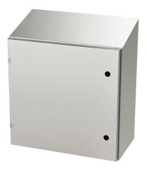
Saginaw Enviroline series enclosure, slope top, NEMA 3R/4/4X/12/13, 24 x 24 x 12in (HxWxD), wall mount, 304 stainless steel, #4 brush finish, single-door, 1/4-turn semi-flush latch.
