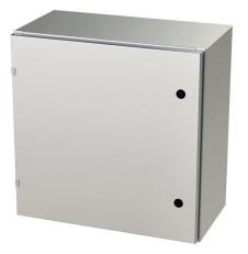
Saginaw Enviroline series enclosure, NEMA 3R/4/4X/12/13,  $24 \times 24 \times 12$ in (HxWxD), wall mount, 304 stainless steel, #4 brush finish, single-door, 1/4-turn semi-flush latch.
