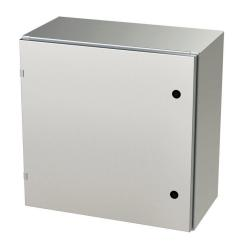
Saginaw Enviroline series enclosure, NEMA 3R/4/4X/12/13, 24 x 24 x 12in (HxWxD), wall mount, 316L stainless steel, #4 brush finish, single-door, 1/4-turn semi-flush latch.
