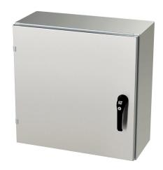
Saginaw Enviroline series enclosure, NEMA 3R/4/4X/12/13, 24 x 24 x 10in (HxWxD), wall mount, 316L stainless steel, #4 brush finish, single-door, 3-point keylocking/padlocking combo handle.
