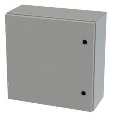
Saginaw Enviroline series enclosure, NEMA 3R/4/12/13, 24 x 24 x 10in (HxWxD), wall mount, carbon steel, ANSI 61 gray, powder coat finish, single-door, 1/4-turn semi-flush latch.
