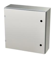
Saginaw Enviroline series enclosure, NEMA 3R/4/4X/12/13,  $24 \times 24 \times 8$  in (HxWxD), wall mount, 304 stainless steel, #4 brush finish, single-door, 1/4-turn semi-flush latch.
