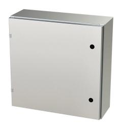
Saginaw Enviroline series enclosure, NEMA 3R/4/4X/12/13, 24 x 24 x 8in (HxWxD), wall mount, 316L stainless steel, #4 brush finish, single-door, 1/4-turn semi-flush latch.
