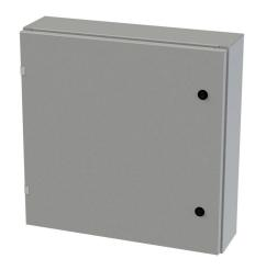
Saginaw Enviroline series enclosure, NEMA 3R/4/12/13,  $24 \times 24 \times 6$  in (HxWxD), wall mount, carbon steel, ANSI 61 gray, powder coat finish, single-door, 1/4-turn semi-flush latch.
