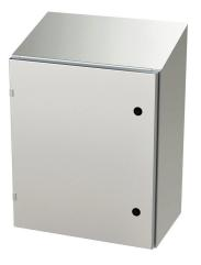
Saginaw Enviroline series enclosure, slope top, NEMA 3R/4/4X/12/13, 24 x 20 x 12in (HxWxD), wall mount, 304 stainless steel, #4 brush finish, single-door, 1/4-turn semi-flush latch.
