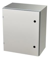
Saginaw Enviroline series enclosure, NEMA 3R/4/4X/12/13,  $24 \times 20 \times 12$ in (HxWxD), wall mount, 304 stainless steel, #4 brush finish, single-door, 1/4-turn semi-flush latch.
