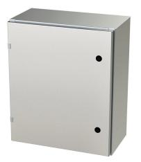
Saginaw Enviroline series enclosure, NEMA 3R/4/4X/12/13, 24 x 20 x 10in (HxWxD), wall mount, 304 stainless steel, #4 brush finish, single-door, 1/4-turn semi-flush latch.
