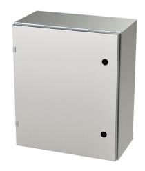
Saginaw Enviroline series enclosure, NEMA 3R/4/4X/12/13, 24 x 20 x 10in (HxWxD), wall mount, 316L stainless steel, #4 brush finish, single-door, 1/4-turn semi-flush latch.
