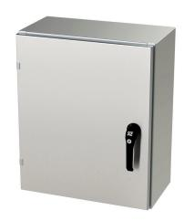
Saginaw Enviroline series enclosure, NEMA 3R/4/4X/12/13,  $24 \times 20 \times 10$  in (HxWxD), wall mount, 316L stainless steel, #4 brush finish, single-door, 3-point keylocking/padlocking combo handle.
