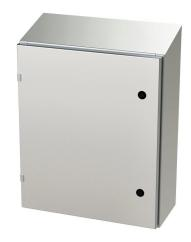
Saginaw Enviroline series enclosure, slope top, NEMA 3R/4/4X/12/13,  $24 \times 20 \times 8$  in (HxWxD), wall mount, 304 stainless steel, #4 brush finish, single-door, 1/4-turn semi-flush latch.
