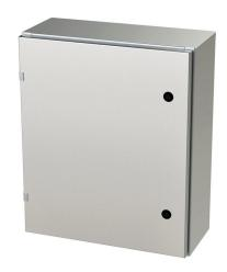
Saginaw Enviroline series enclosure, NEMA 3R/4/4X/12/13,  $24 \times 20 \times 8$  in (HxWxD), wall mount, 316L stainless steel, #4 brush finish, single-door, 1/4-turn semi-flush latch.
