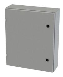
Saginaw Enviroline series enclosure, NEMA 3R/4/12/13,  $24 \times 20 \times 6$  in (HxWxD), wall mount, carbon steel, ANSI 61 gray, powder coat finish, single-door, 1/4-turn semi-flush latch.
