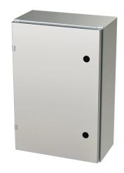
Saginaw Enviroline series enclosure, NEMA 3R/4/4X/12/13,  $24 \times 16 \times 8$  in (HxWxD), wall mount, 304 stainless steel, #4 brush finish, single-door, 1/4-turn semi-flush latch.
