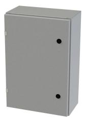
Saginaw Enviroline series enclosure, NEMA 3R/4/12/13,  $24 \times 16 \times 8in$  (HxWxD), wall mount, carbon steel, ANSI 61 gray, powder coat finish, single-door, 1/4-turn semi-flush latch.
