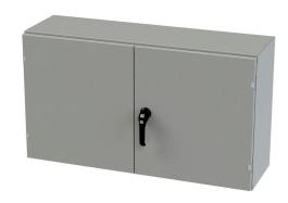
Saginaw enclosure, NEMA 3R/12/13, 24 x 42 x 12in (HxWxD), wall mount, carbon steel, ANSI 61 gray, powder coat finish, doubledoor, 3-point keylocking/padlocking combo handle.
