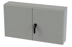
Saginaw enclosure, NEMA 3R/12/13, 24 x 42 x 8in (HxWxD), wall mount, carbon steel, ANSI 61 gray, powder coat finish, double-door, 3-point keylocking/padlocking combo handle.
