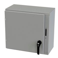
Saginaw Enviroline series disconnect enclosure, NEMA 3R/4/12/13, right flange, 20 x 21 x 10in (HxWxD), wall mount, carbon steel, ANSI 61 gray, powder coat finish, single-door, 2-point padlocking handle, purchase subpanel separately.
