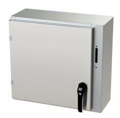
Saginaw Enviroline series disconnect enclosure, NEMA 3R/4/4X/12/13, right flange, 20 x 21 x 8in (HxWxD), wall mount, 304 stainless steel, #4 brush finish, single-door, 2-point padlocking handle, purchase subpanel separately.
