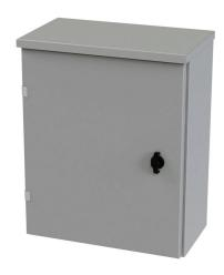
Saginaw enclosure, NEMA 3R, 20 x 16 x 8in (HxWxD), wall mount, carbon steel, ANSI 61 gray, powder coat finish, single-door, 1/4-turn padlocking wing handle.
