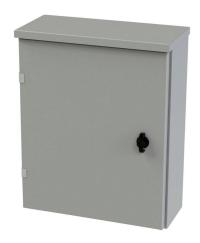
Saginaw enclosure, NEMA 3R, 20 x 16 x 6in (HxWxD), wall mount, carbon steel, ANSI 61 gray, powder coat finish, single-door, 1/4-turn padlocking wing handle.
