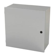
Saginaw enclosure, NEMA 1, 20 x 20 x 10in (HxWxD), wall mount, carbon steel, ANSI 61 gray, powder coat finish, single-door, 1/4-turn semi-flush latch.
