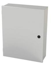
Saginaw enclosure, NEMA 1, 20 x 16 x 6in (HxWxD), wall mount, carbon steel, ANSI 61 gray, powder coat finish, single-door, 1/4-turn semi-flush latch.
