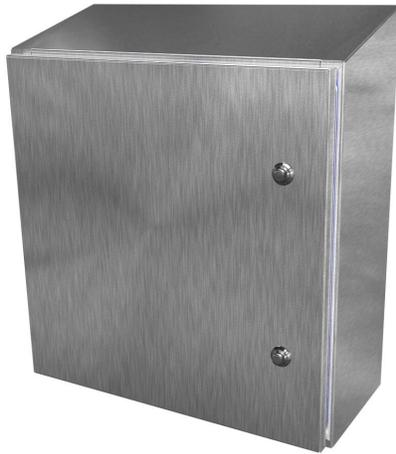
Saginaw sanitary enclosure, slope top, NEMA 3R/4/4X/12, 20 x 20 x 8in (HxWxD), wall mount, 304 stainless steel, #4 brush finish, single-door, 1/4-turn sanitary stainless steel latch.
