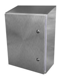
Saginaw sanitary enclosure, slope top, NEMA 3R/4/4X/12, 20 x 16 x 8in (HxWxD), wall mount, 304 stainless steel, #4 brush finish, single-door, 1/4-turn sanitary stainless steel latch.
