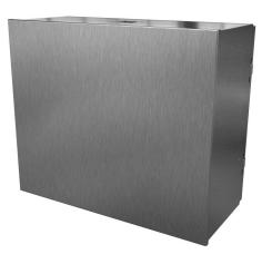
Saginaw HMI Enclosure, NEMA 3R/4/4X/12/13, 20 x 24 x 10in (HxWxD), suspension or pedestal mount, dual access, 304 stainless steel, #4 brush finish, screw cover front, single door rear, 1/4-turn semi-flush latch.
