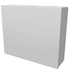
Saginaw HMI Enclosure, NEMA 3R/4/12/13, 20 x 24 x 6in (HxWxD), suspension or pedestal mount, dual access, carbon steel, RAL 7035 light gray, powder coat finish, screw cover front, single door rear, 1/4-turn semi-flush latch.
