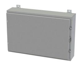
Saginaw enclosure, NEMA 3R/4/12/13, 20 x 30 x 6in (HxWxD), wall mount, carbon steel, ANSI 61 gray, powder coat finish, single-door, plated steel clamps, padlock hasp and staple.
