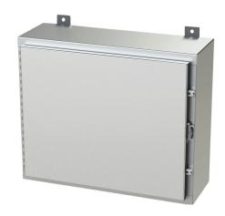
Saginaw enclosure, NEMA 3R/4/4X/12/13, 20 x 24 x 8in (HxWxD), wall mount, 304 stainless steel, #4 brush finish, single-door, stainless steel clamps, padlock hasp and staple.
