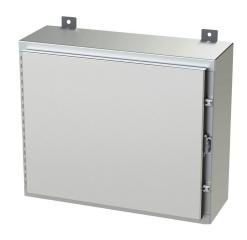
Saginaw enclosure, NEMA 3R/4/4X/12/13, 20 x 24 x 8in (HxWxD), wall mount, 316L stainless steel, #4 brush finish, single-door, stainless steel clamps, padlock hasp and staple.
