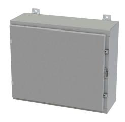
Saginaw enclosure, NEMA 3R/4/12/13, 20 x 24 x 8in (HxWxD), wall mount, carbon steel, ANSI 61 gray, powder coat finish, single-door, plated steel clamps, padlock hasp and staple.
