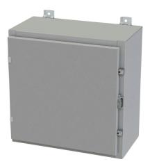
Saginaw enclosure, NEMA 3R/4/12/13, 20 x 20 x 10in (HxWxD), wall mount, carbon steel, ANSI 61 gray, powder coat finish, single-door, plated steel clamps, padlock hasp and staple.
