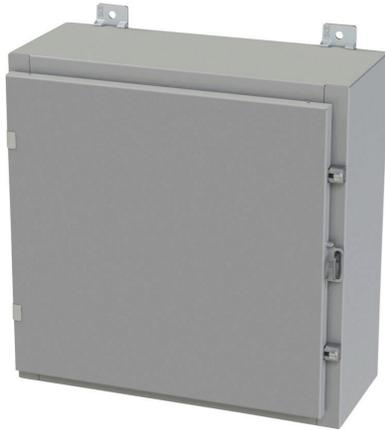
Saginaw enclosure, NEMA 3R/4/12/13, 20 x 20 x 8in (HxWxD), wall mount, carbon steel, ANSI 61 gray, powder coat finish, single-door, plated steel clamps, padlock hasp and staple.
