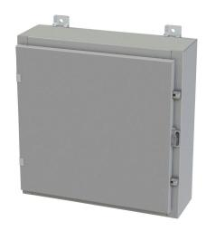
Saginaw enclosure, NEMA 3R/4/12/13, 20 x 20 x 6in (HxWxD), wall mount, carbon steel, ANSI 61 gray, powder coat finish, single-door, plated steel clamps, padlock hasp and staple.
