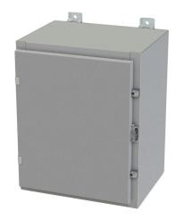
Saginaw enclosure, NEMA 3R/4/12/13, 20 x 16 x 12in (HxWxD), wall mount, carbon steel, ANSI 61 gray, powder coat finish, single-door, plated steel clamps, padlock hasp and staple.
