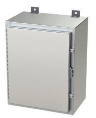
Saginaw enclosure, NEMA 3R/4/4X/12/13, 20 x 16 x 10in (HxWxD), wall mount, 304 stainless steel, #4 brush finish, single-door, stainless steel clamps, padlock hasp and staple.
