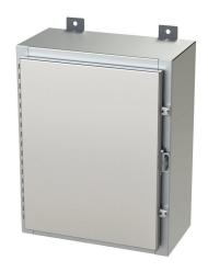
Saginaw enclosure, NEMA 3R/4/4X/12/13, 20 x 16 x 8in (HxWxD), wall mount, 304 stainless steel, #4 brush finish, single-door, stainless steel clamps, padlock hasp and staple.
