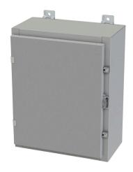
Saginaw enclosure, NEMA 3R/4/12/13, 20 x 16 x 8in (HxWxD), wall mount, carbon steel, ANSI 61 gray, powder coat finish, single-door, plated steel clamps, padlock hasp and staple.
