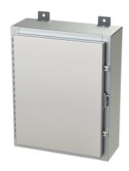
Saginaw enclosure, NEMA 3R/4/4X/12/13, 20 x 16 x 6in (HxWxD), wall mount, 316L stainless steel, #4 brush finish, single-door, stainless steel clamps, padlock hasp and staple.
