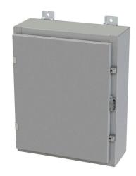
Saginaw enclosure, NEMA 3R/4/12/13, 20 x 16 x 6in (HxWxD), wall mount, carbon steel, ANSI 61 gray, powder coat finish, single-door, plated steel clamps, padlock hasp and staple.
